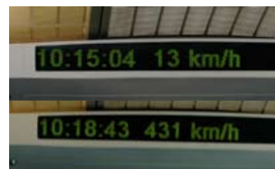
The times and the speed of the train. It took less than 4 minutes for the train to get up to maximum speed!
